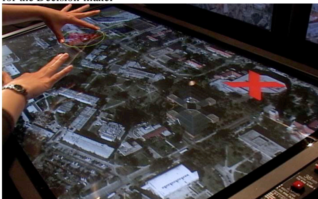
Figure 2.3 Polyphonic touch-display created at the UF Digital Worlds Institute allows Operator to quickly select and interact with target areas
