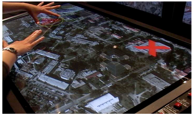
Figure 2.3 Polyphonic touch-display created at the UF Digital Worlds Institute allows Operator to quickly select and interact with target areas
